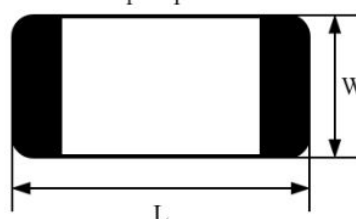
贴片电容 Chip Capacitor
